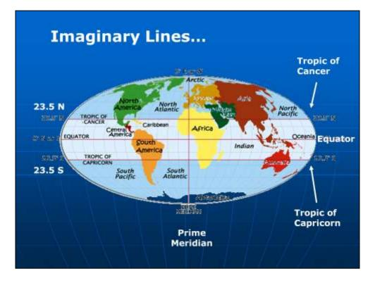
**Distance between Lines** If you divide the circumference of the earth (*approximately 25,000 miles*) by 360 degrees, the distance on the earth's surface for each one degree of latitude or longitude is just over 69 miles, or 111 km. **Note:** As you move north or south of the equator, the distance between the lines of longitude gets shorter until they actually meet at the poles. At 45 degrees N or S of the equator, one degree of longitude is about 49 miles.
