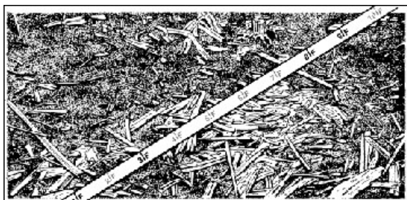
Figure 1 Lay out a 100-foot tape measure across crop rows at a 45-degree diagonal. Anchor both ends in a row. Look straight down at each 1-foot mark, always choosing the same side of the tape. Count the number of times that a piece of crop residue intersects the tape measure at one of the 1-foot marks. Example: the 1-, 3-, 8- and 9-foot markers have residue, while the 2-, 4-, 5-, 6-, 7- and 10-foot markers do not have residue.
