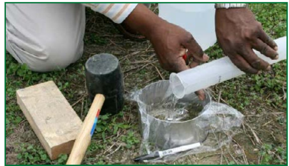
Figure 2.—Water is poured into plastic-lined ring.
