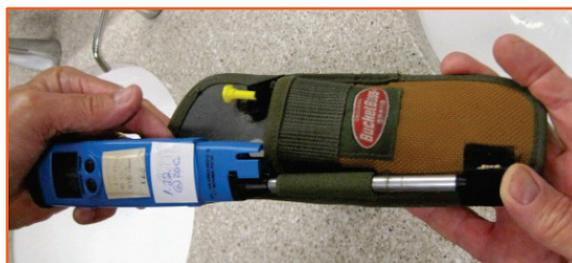
Figure 2.—EC probe inserted into resistor on holster to check calibration (Doran and Kucera, 2012).
