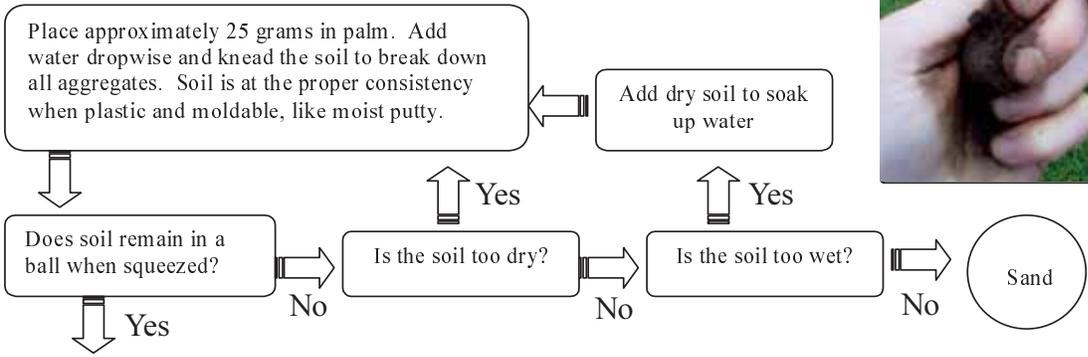
Place ball of soil between thumb and forefinger, gently push the soil with the thumb, squeezing it upward into a ribbon. Form a ribbon of uniform thickness and width. Allow the ribbon to emerge and extend over the forefinger, breaking from its own weight.
