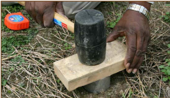
Figure 6.—Drive ring into soil to a depth of 3 inches.
