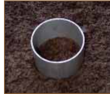
Figure 7.—Ring extends 2 inches above the surface.
