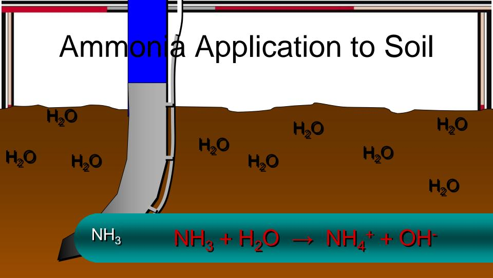
Ammonium (NH<sub>4</sub><sup>+</sup>) binds rapidly to cation exchange sites on soil clay particles and soil organic matter. Hydroxyl anions effectively increase soil pH.
