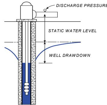
Figure 1. Pumping lift and location of discharge pressure.
